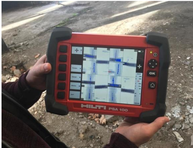
Fig. 5. Examination of carrying elements with X-ray device.
