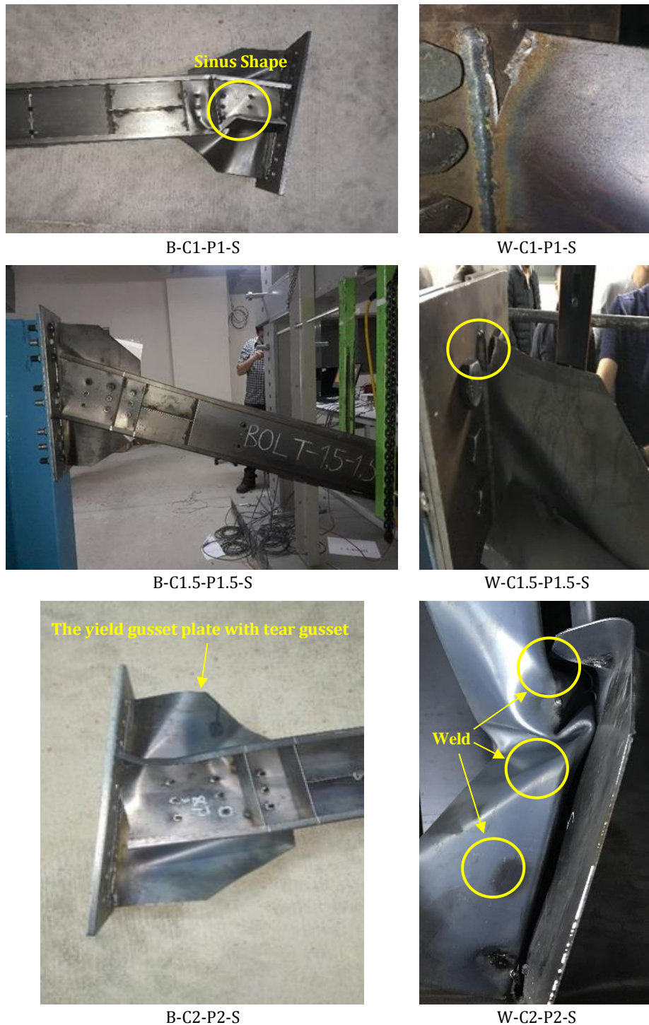
Fig. 6. Collapse modes of test specimens and comparing collapse mode.
