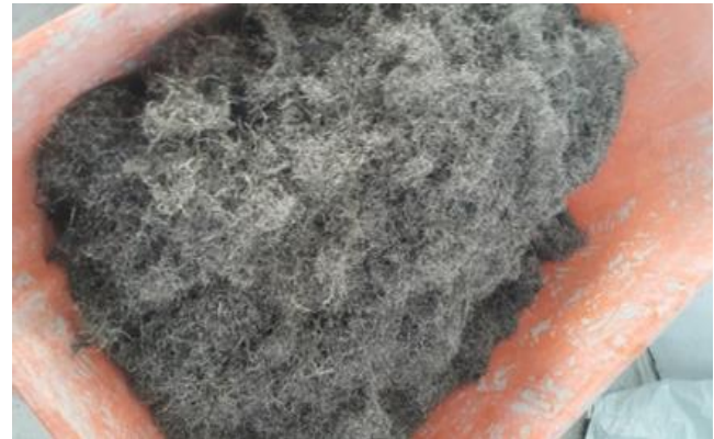
Fig. 1. Waste steel tire wire sample used for tests.
