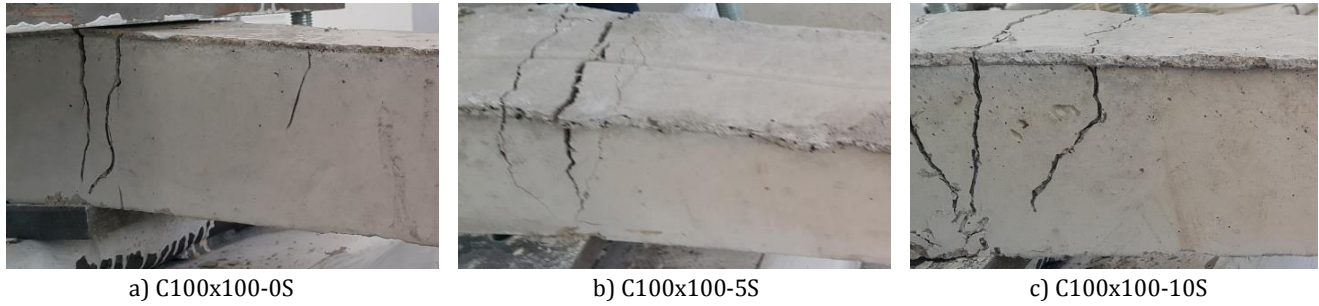
Fig. 11. Failure of the C100x100 concrete bollards under impact loading.
