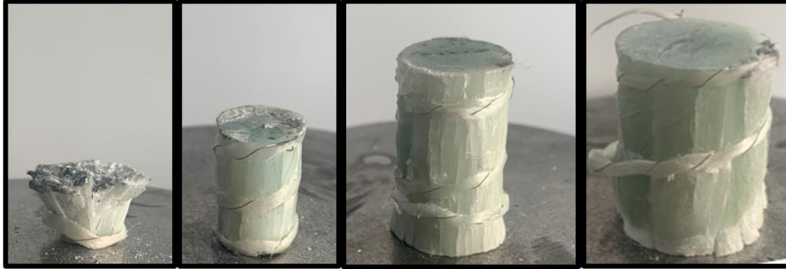
Fig. 3. Specimen images after compression test.
