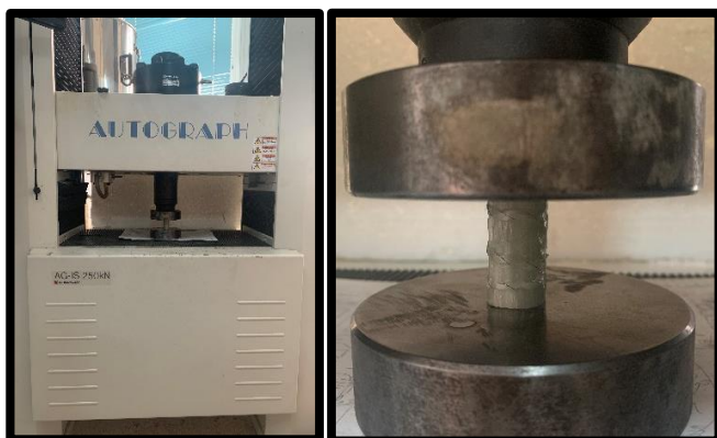
Fig. 2. Compression test apparatus and GFRP specimen.
