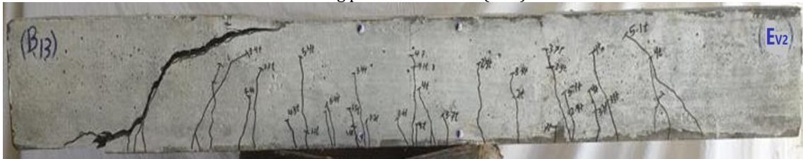
Cracking patterns for beam (EV2)
