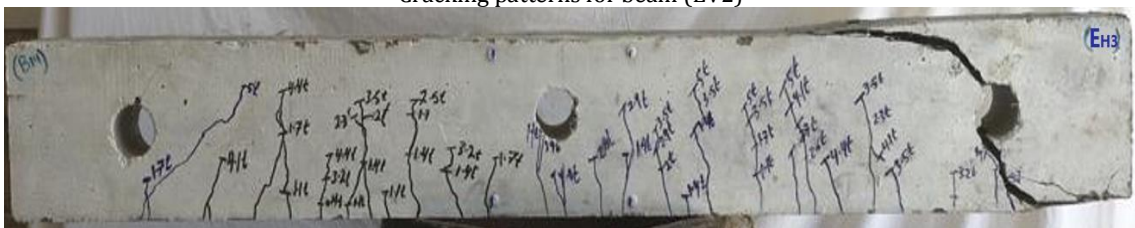
Cracking patterns for beam (EH3)
