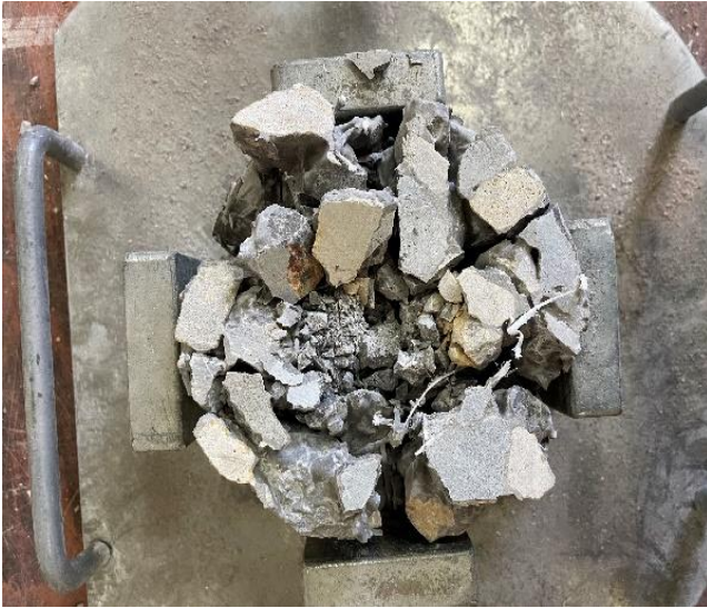
Fig. 14. Crack pattern at total fracture.
