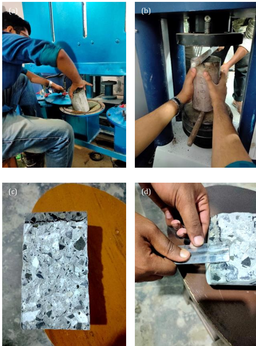
Fig. 11. Water permeability test procedure: (a) Specimen placing; (b) Splitting; (c) Marking; (d) Measuring.
