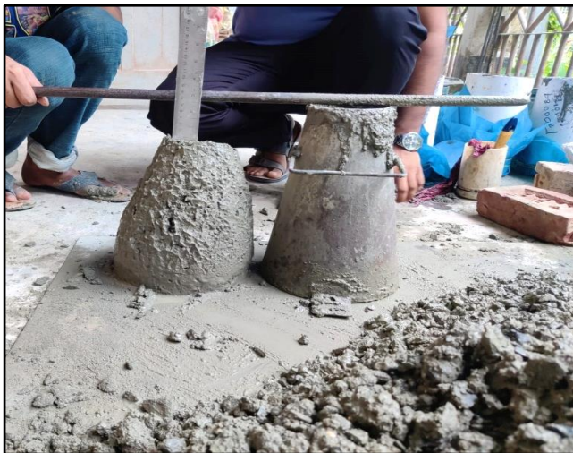
Fig. 6. Measuring the slump value of the concrete mix.
