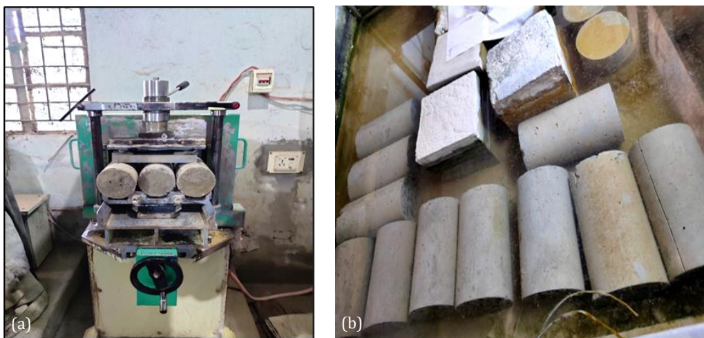
Fig. 7. (a) Cutting of specimen; (b) Ponding method for curing of specimen.
