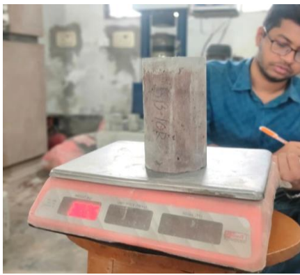
Fig. 8. The load-measuring method of the test specimen.
