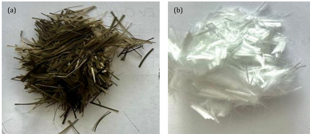
Fig. 1. View of fibers: (a) Basalt fibers; (b) Polypropylene fibers.
