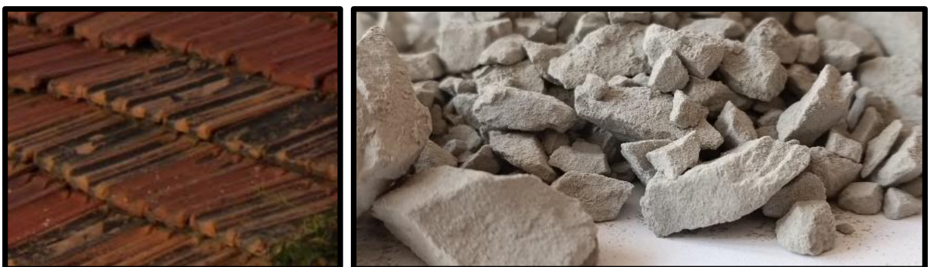
Fig. 1. Expired cement and aged roof tile.
