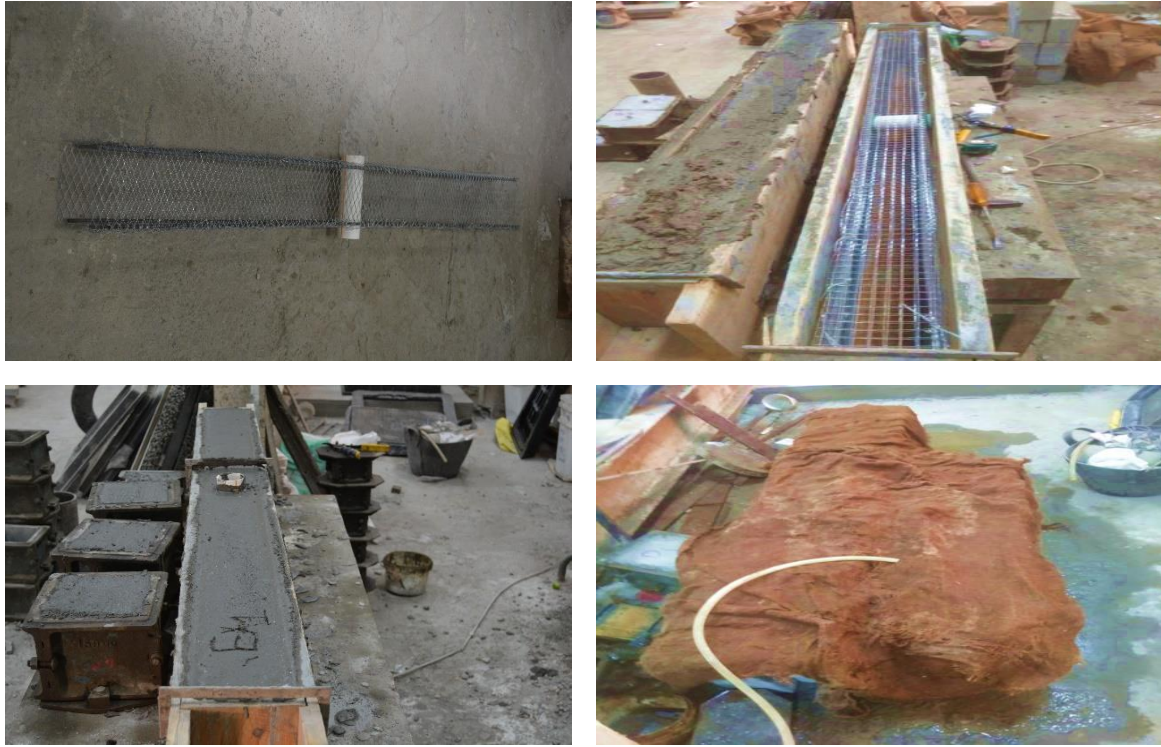
Fig. 4. Phases of specimen preparation until the casting and curing process.
