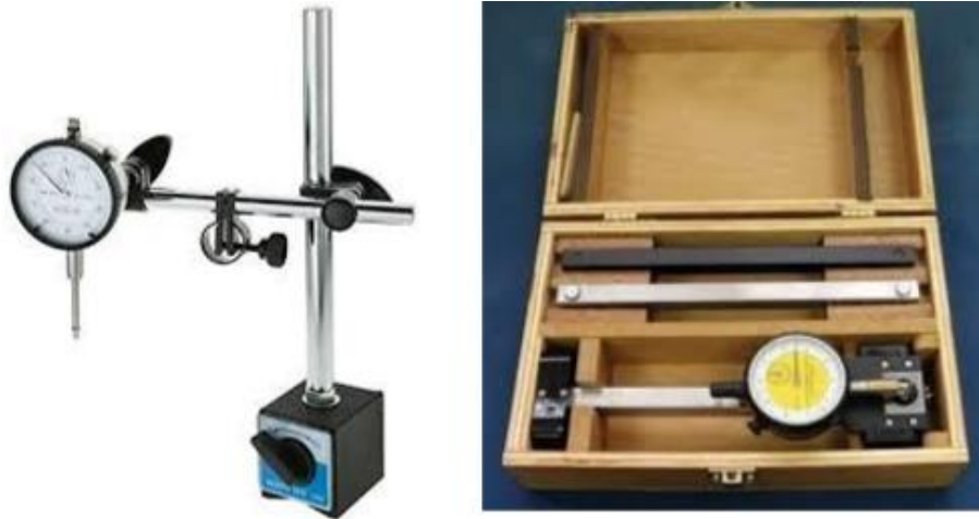
Fig. 6. The dial gauge and deflection gauge used in the study.
