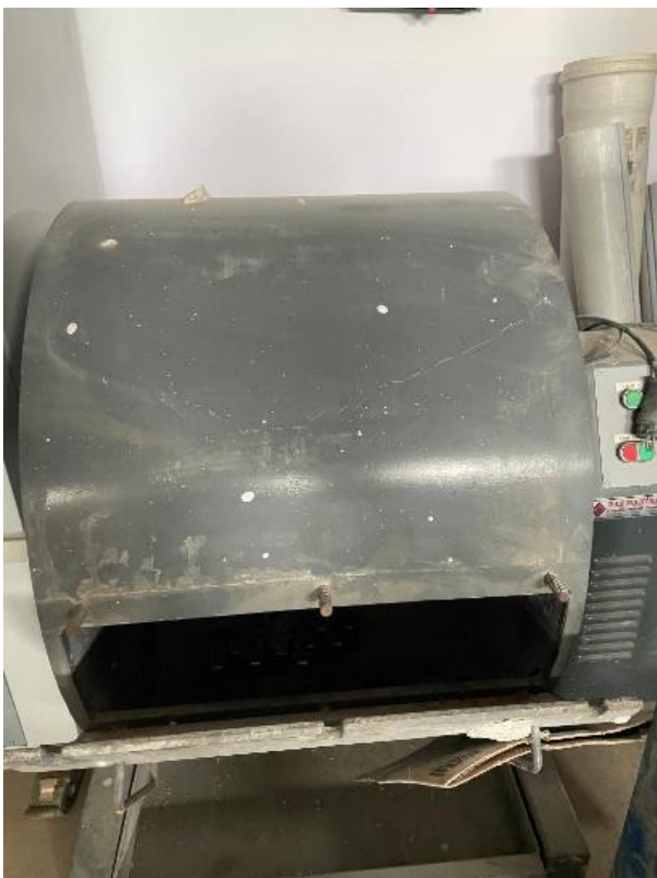
Fig. 5. Abrasion resistance test setup.
