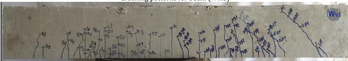
Cracking patterns for beam (Wv3) (b) Beams of the Group B with welded mesh.
