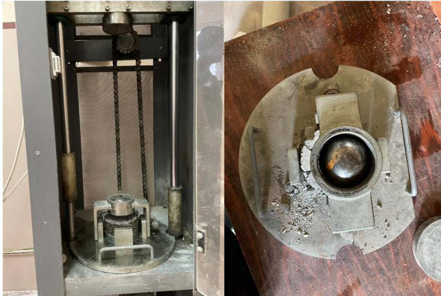
Fig. 4. Impact resistance test setup.
