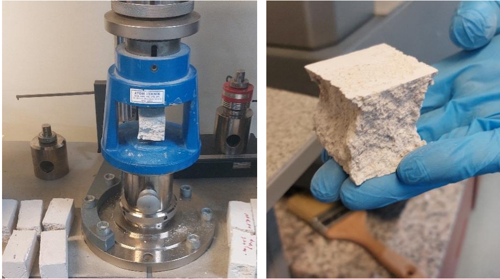
Fig. 12. Compression test on the specimens.
