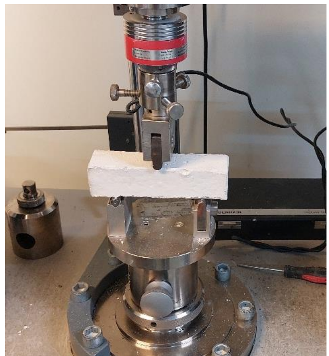
Fig. 11. Three-point bending test on the specimens.
