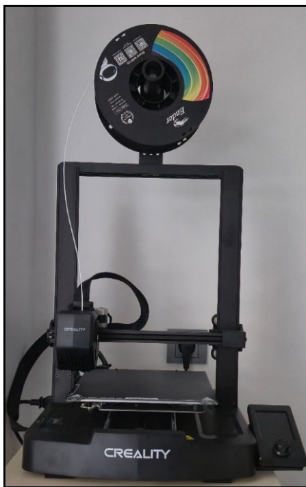
Fig. 1. FDM 3D printer used in the production of experimental samples.
