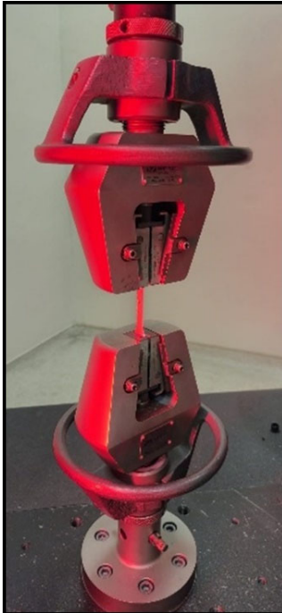
Fig. 6. The image of experimental samples in the tensile test device.
