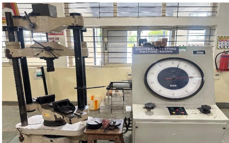
Fig. 7. Test setup for pull-out test.
