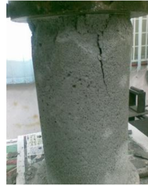
Fig. 3. Concrete cracking pattern in 28 days compressive strength test.
