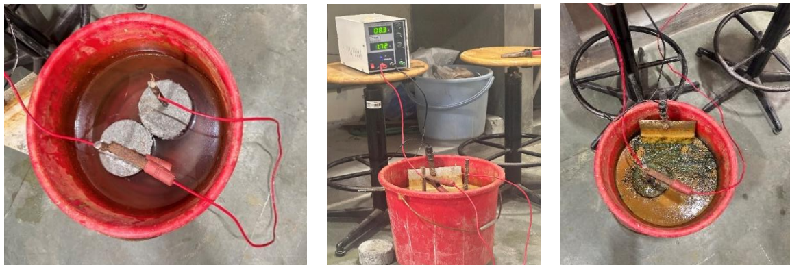
Fig. 6. Accelerated corrosion test setup.
