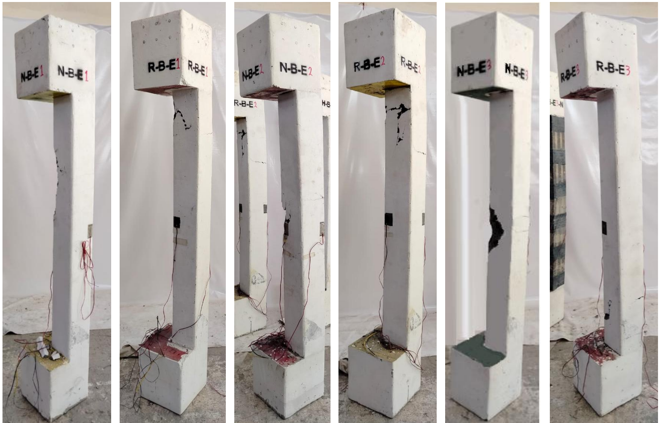
Fig. 16. Observed failure modes of the tested specimens.
