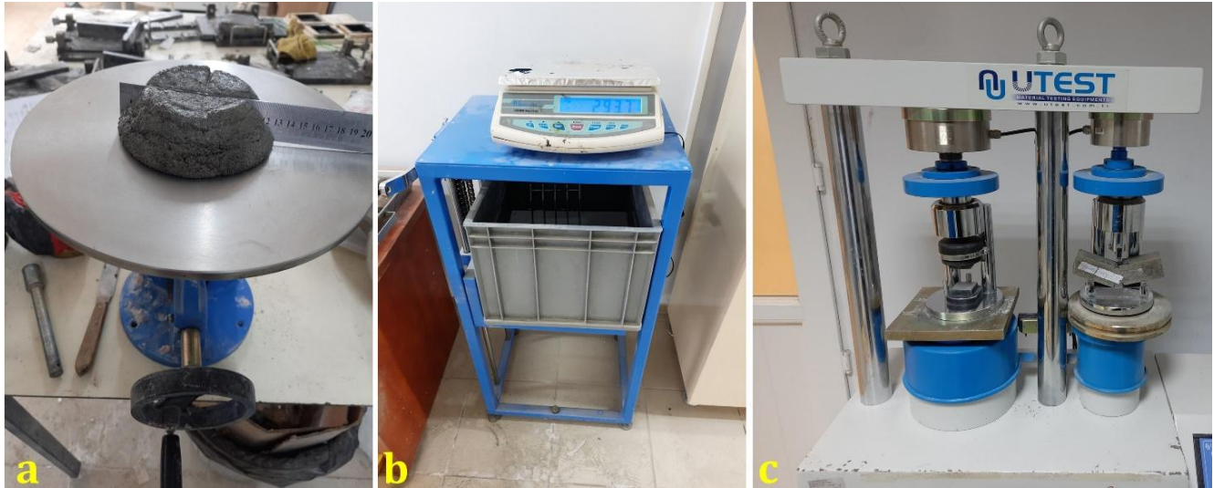
Fig. 3. Experimental test setups used for evaluating mortar properties: (a) Flow table apparatus; (b) Archimedes balance; (c) Flexural/compressive strength testing machine.
