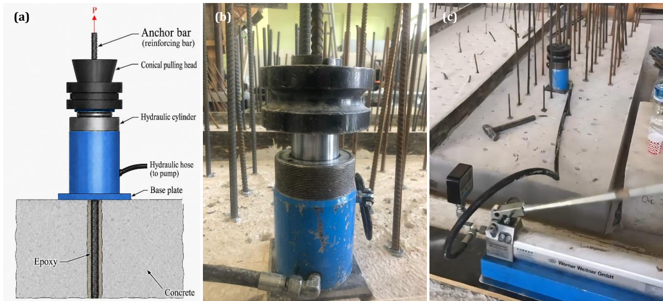
Fig. 3. Pull-out test: (a) Modeling; (b) Hydraulic cylinder setup; (c) Experimental setup.
