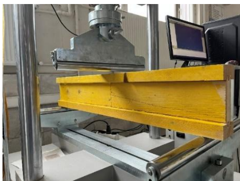
Fig. 5. Three-point bending test setup showing the midspan load, simply supported boundary conditions, clear support span ( L = 1000 \text{ mm} ), and beam depth ( h ).
