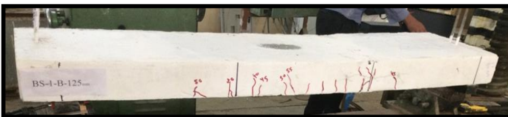
(e) Flexural failure of (BS-1-B-125mm)
