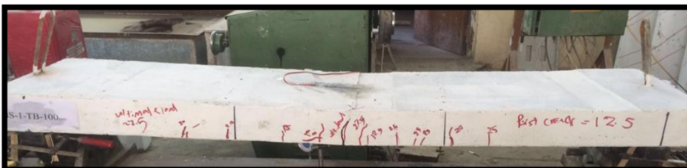
(f) Flexural failure of (S-1-TB-100mm)
