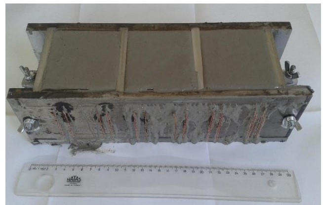
Fig. 3. Mix casted in mold.
