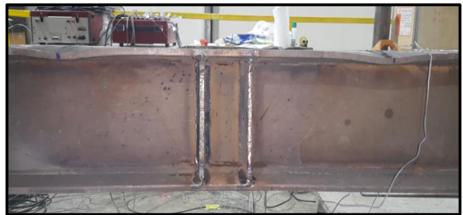
Fig. 19. Buckling of a beam compression flange.
