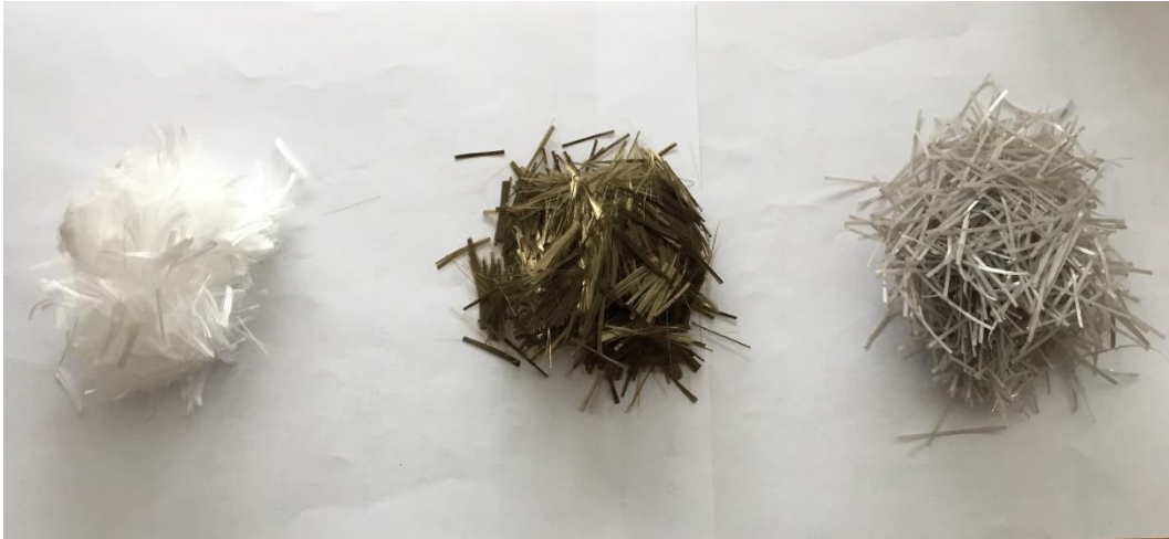
Fig. 1. Polypropylene, basalt and macro-synthetic fibre.
