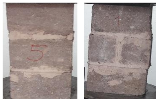
Fig. 3. Experimental assemblage samples with Khorasan mortar.
