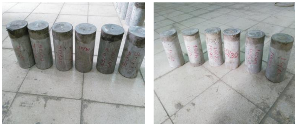
Fig. 5. Siliconization of the samples to be tested for capillarity.
