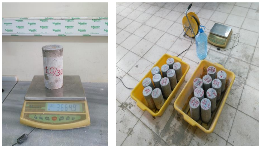
Fig. 7. Measurement of mass changes at the specified time in the capillary test apparatus.
