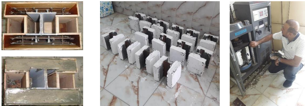
Fig. 7. Fabrication, casting, and testing of push-out specimens.
