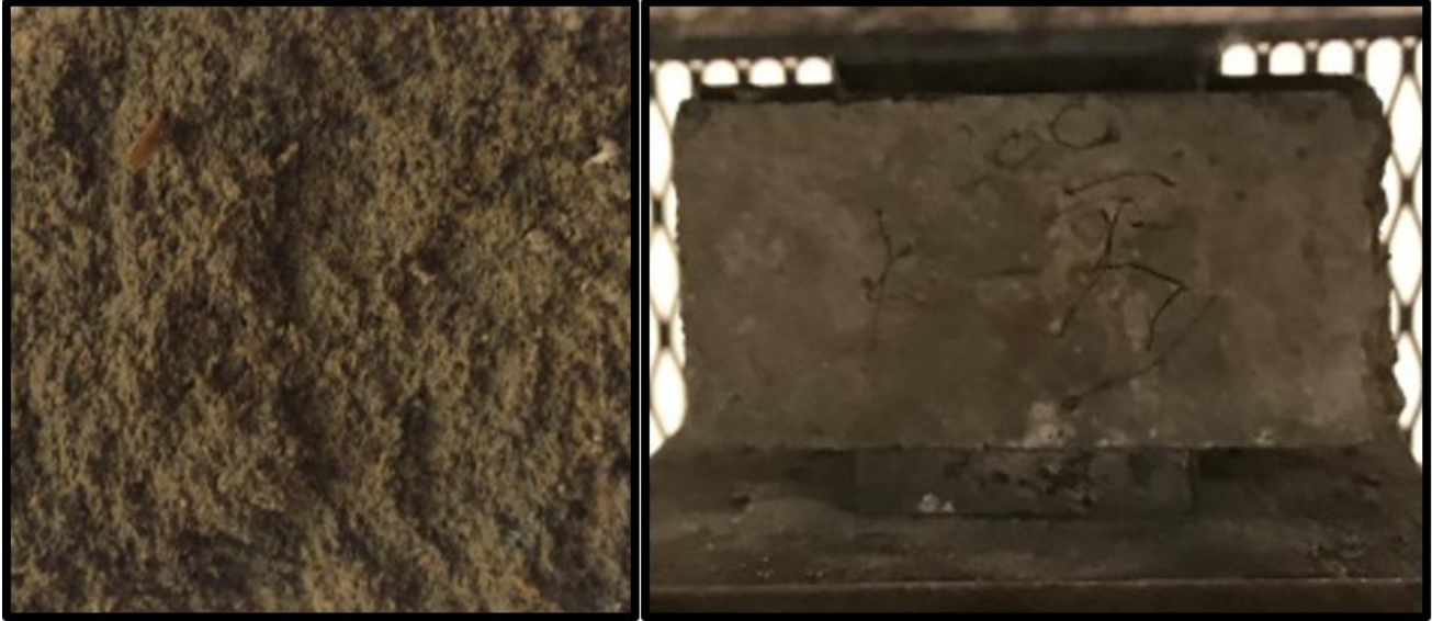
Fig. 3. Cement-bonded wood mixtures and compressive test.
