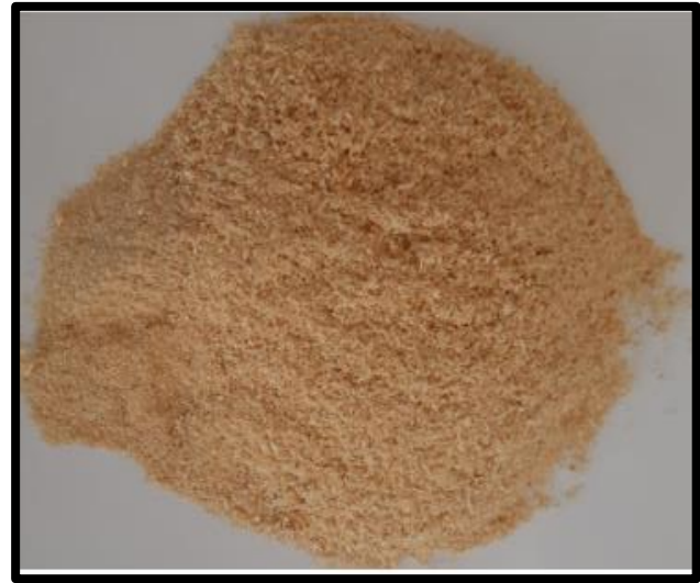
Fig. 2. The sawdust used in the production of cement-bonded composite.
