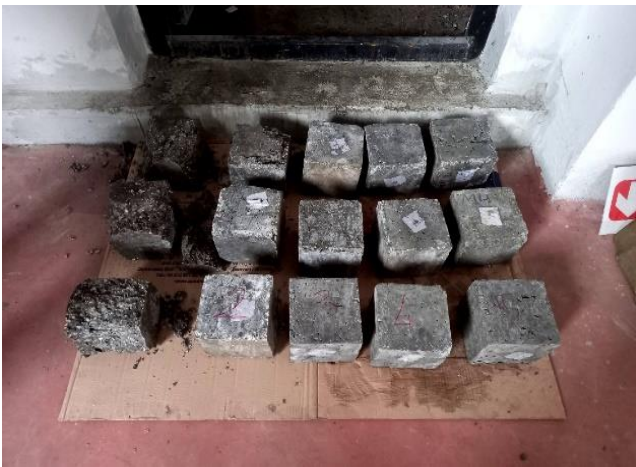
Fig. 10. View of all concrete samples subjected to compressive strength test (for 7 days).
