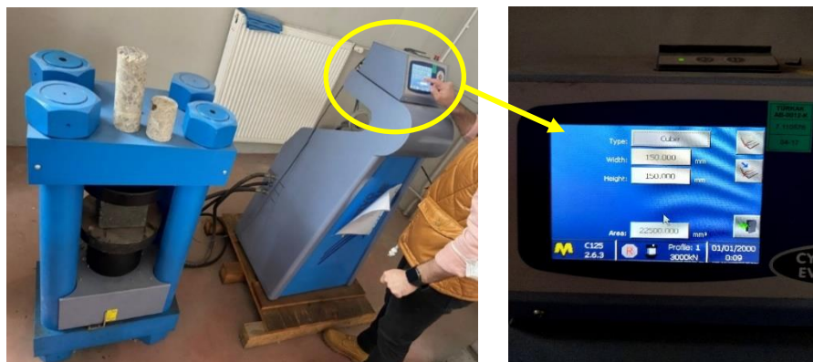
Fig. 8. Using the compressive strength device.
