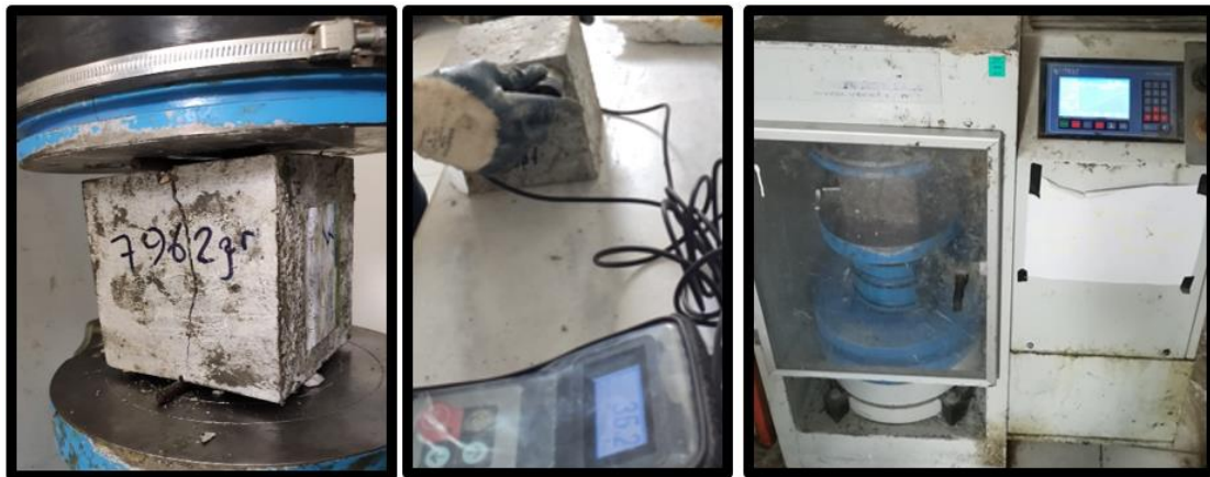
Fig. 4. Ultrasonic pulse velocity and mechanical tests.
