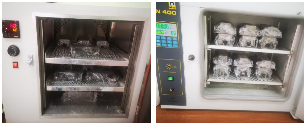
Fig. 4. 30 °C and 60 °C heat curing of PGC samples.
